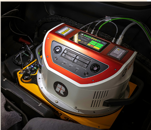
RIEGL VQ-1260 installed on the GSM-4000 gyro-stabilized platform
